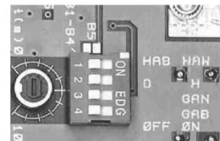
Use the potentiometer to the left of the switches to set the GAN and GAB times steplessly from 0.1 s ... 10 s.
